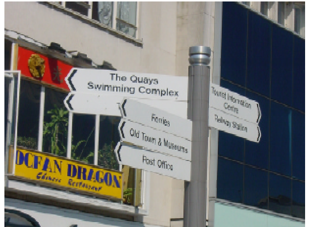
Contemporary stainless steel finger posts look attractive and are easily maintained, however the 'shot-peened' finish is not easy to maintain
